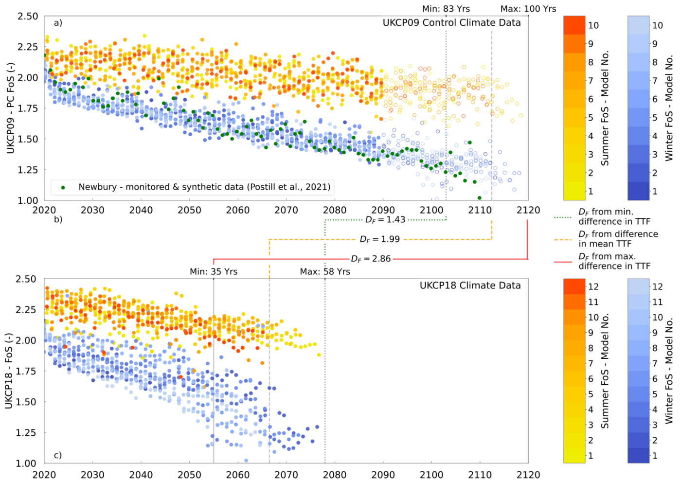
Figure 2: a) UKCP09 control (no-change) climate-driven factor of safety (FoS) deterioration curves; b) deterioration factors, D_f , calculated for the high plasticity clay cut slope numerical models from time to failure (TTF); c) FoS deterioration curves driven by the 12 UKCP18 RCP8.5 regional climate model perturbed parameter ensembles (future climate change). [16]
